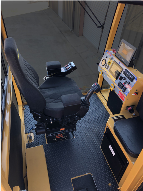
Spartan control panel and operational controls.
