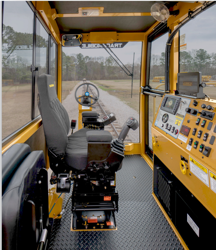
Titan control panel and operational controls.
